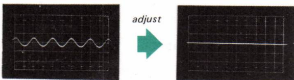
Fig. 3-8. Fm discriminator alignment output response
